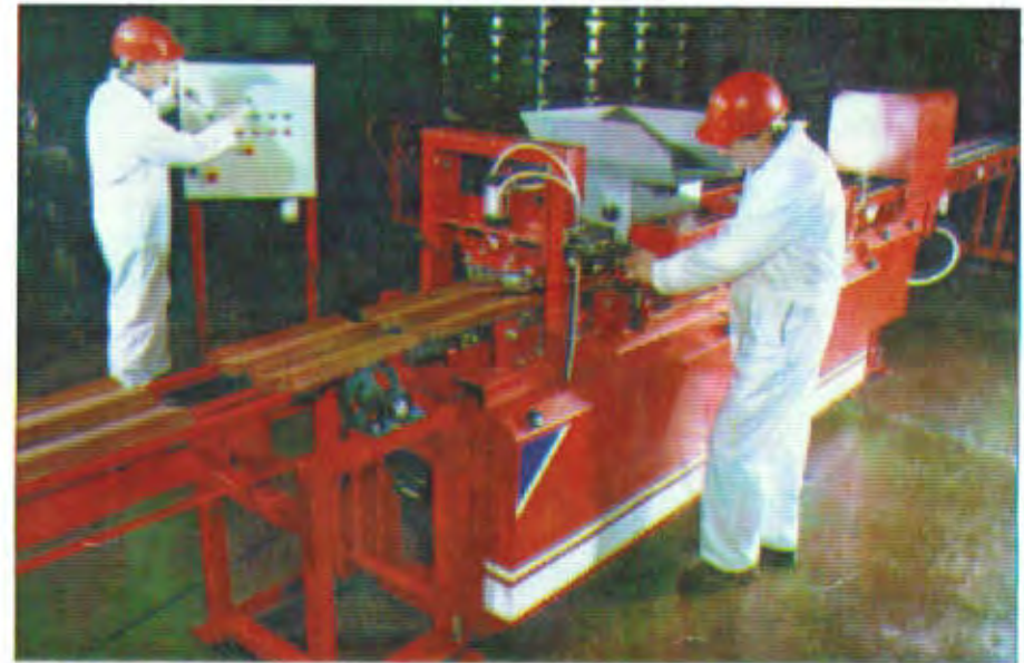
Annith 15 - Tile extrusion machine with electrical control panel in background
