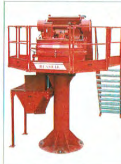
Concrete batching and mixing plant
